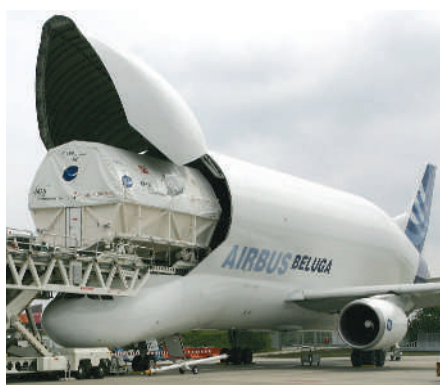
Hitching a lift: the European space lab Columbus went by plane to NASA's Kennedy Space Center.
